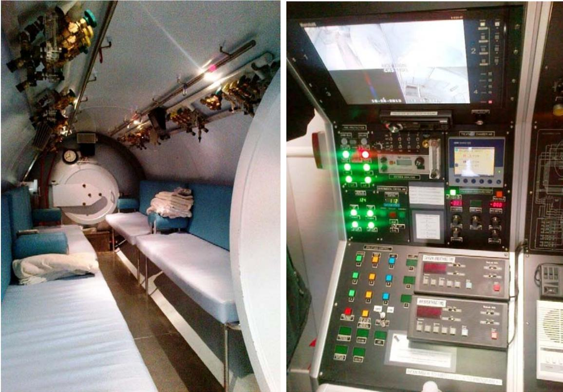
**(Above, left)** The roomy interior of the hyperbaric chamber; **(Above, right)** The chamber's control console.
