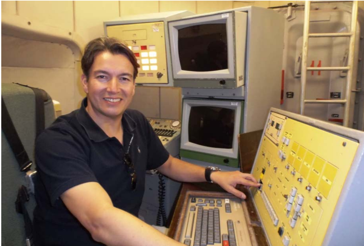
(Above) Deep underground, in the 11 th section of the launch command center, A.C. Frieden sits at the launch operator's chair, with the missile launch key and button activated. The monitors, communications gear and launch code vault to his left comprise the secure launch order verification system that would have been crucial had a missile strike been ordered from Moscow.
