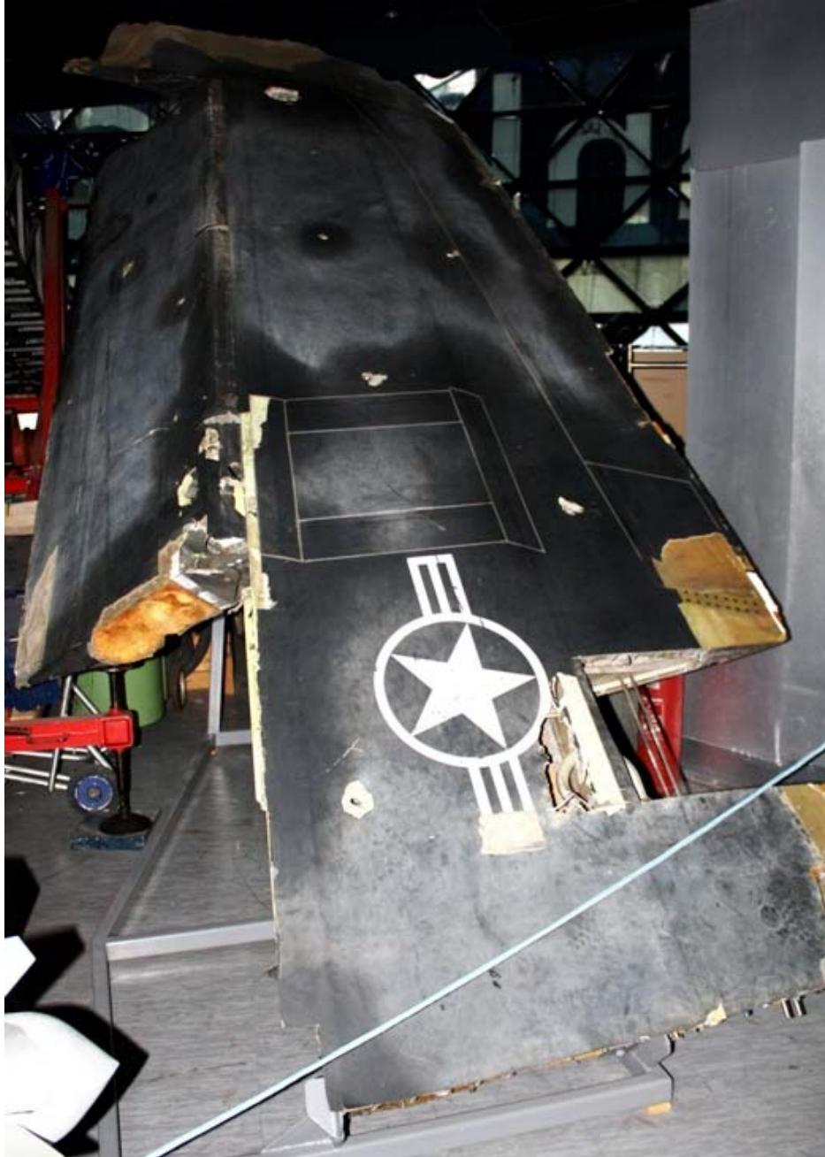
Photo above: A large section of the U.S. F-117A Nighthawk's port wing, including the outer flaps and leading edge assembly, is on display at Belgrade's Aviation Museum.
